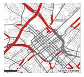
Center City Level of Service (red indicates a failing LOS of E or F).
